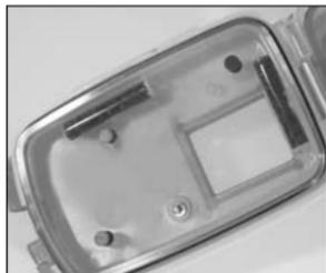
Prevent fogging keep camera power off as much as possible. Use Moisture Muncher desiccant capsules. Apply anti-fog to inside of lens port. Keep inside of housing perfectly dry. Seal housing in a dry, air conditioned room. Insert Moisture Muncher in holding area as shown. Replace when capsules turn pink.
