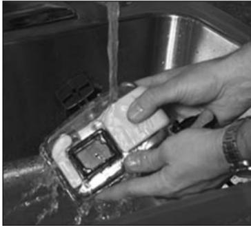
**Soak the sealed housing in fresh water immediately after every dive.** This will dissolve any salt and clean off dirt and sand. Most dive boats have a fresh water bucket for cameras. Push and release several times every button on the housing to rinse out the sand and salt water. Do not use the mask bucket because this is full of detergents. Never use any detergents, cleaners or chemicals to clean the camera. Dry the housing before opening.
