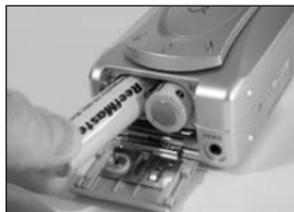
Use freshly charged SeaLife Ni-MH AA batteries (2100mAh or higher). Save battery power by keeping camera or power off whenever possible. Use SeaLife AC Adaptor - Item# SL932 for continuous power. Use of DC100/D200 or other A/C adaptors will cause damage to camera.
