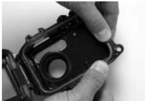
**Step 4: Carefully close housing to firmly seat O-ring and open housing again to inspect that O-ring is completely seated into groove. Do NOT grease the O-ring.**
