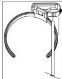
**Step 2: Use small wrench provided to tighten set screw until you feel some resistance. Do not over tighten! Gently pull on cable to check that it is firmly attached.**
