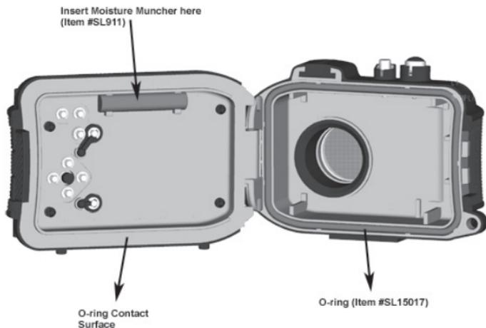
Important: Carefully clean and inspect O-ring and O-ring contact surfaces before each underwater use in accordance with instructions provided in this manual.
