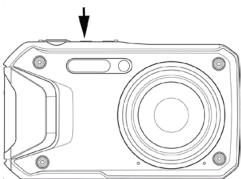
**Note**: Pushing and holding the shutter button halfway will focus the camera on the subject. A green focus box indicates the camera has accurately focused on a subject. A red focus box indicates the camera has NOT accurately focused on a subject. This function is useful for checking that the camera has focused on a subject before shooting.
