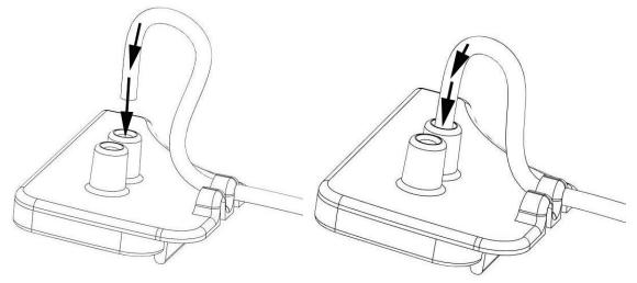
3) Pull the other end of the camera to remove some of the extra slack, leaving about 1" of cable bend as shown below. It is normal for thin layer of cable sheathing to be scratched off during this procedure.
