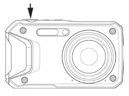
3) **Record a video:** Push the video button ( down to start recording. Push video button again to stop recording.
