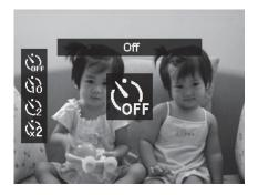
Note: The Self-timer function resets to **Off** after every shot or when powering off the camera.
