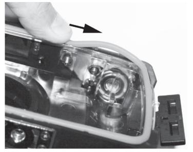
2) Gently pull the O-ring out of its groove.
