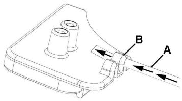
2) Pull about 2" (5cm) of the optical cable through the grabber hole and insert the end of the cable into the other hole as shown below. Push cable end down into the hole until it comes to a stop.
