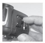
Step 2: Open latch all the way to lift and release latch from housing.
