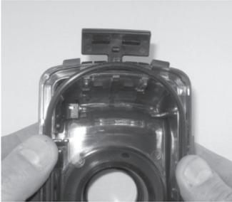
Step 2: Push O-ring into groove as shown being careful not to twist or roll O-ring.
