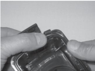
Step 4: Carefully close housing to firmly seat O-ring and open housing again to inspect that O-ring is completely seated into groove. Do NOT grease the O-ring.
