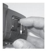
Step 2: Open latch all the way to lift and release latch from housing.
