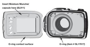
Important: Carefully clean and inspect O-ring and O-ring contact surfaces before each underwater use in accordance with instructions provided in this manual.
