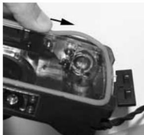
Step 2: Gently lift and remove O-ring from its groove.
