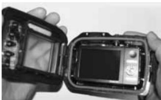
Step 4: Close housing and push down on latch as shown to firmly seat latch into housing.
