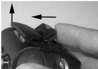
Step 3: Open Housing as shown so inner camera does not fall out.
