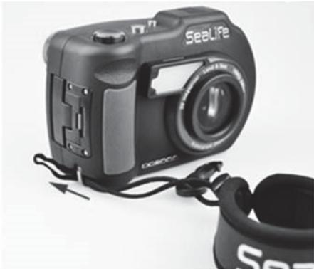
Insert looped end of nylon cord through the housing strap connector.
