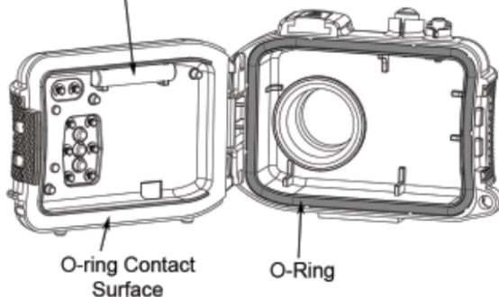
Important: Carefully clean and inspect O-ring and O-ring contact surfaces before each underwater use in accordance with instructions provided in this manual.
