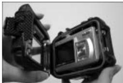
**Step 4: Close housing and push down on latch as shown to firmly seat latch into housing.**
