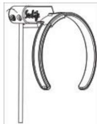
**Step 3: Attach adapter around housing lens port so that it is seated into the flash window recess.**
