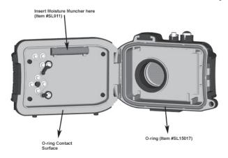
Important: Carefully clean and inspect O-ring and O-ring contact surfaces before each underwater use in accordance with instructions provided in this manual.
