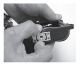
Step 2: Gently lift and remove O-ring from its groove.
