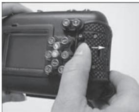
Step 2: Open latch all the way to lift and release latch from housing.
