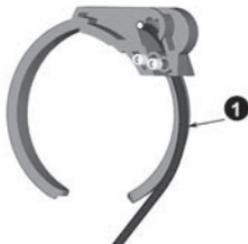
Step 2: Use small wrench provided to tighten set screw until you feel some resistance. Do not over tighten! Gently pull on cable to check that it is firmly attached.
