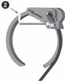
Step 3: Attach adapter around housing lens port so that it is seated into the flash window recess.
