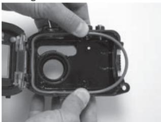
Step 2: Push O-ring into groove as shown being careful not to twist or roll O-ring.
