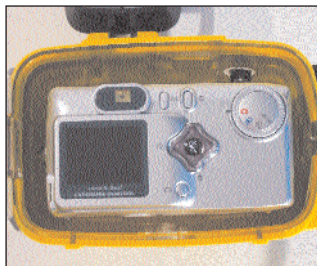
9. Insert camera. Do this in a dry, air-conditioned room or housing may fog.
