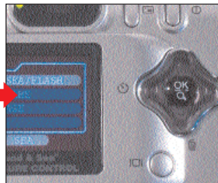
2. Use right arrow NAV button to select SEA mode. Select FLASH only if using External Strobe.
