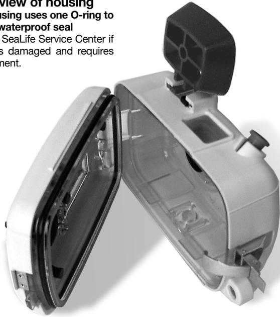
Important: Carefully inspect o-ring for salt, sand, hair, cuts, tears or other damage. Clean o-ring before every use. Replace o-ring if damaged.
