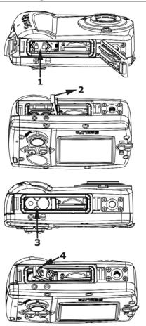
1) Slide battery door cover to unlock position.
