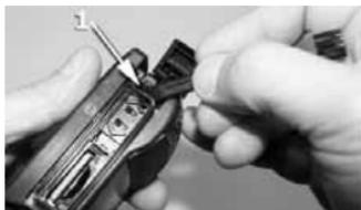
1) Remove the O-ring using the end of the cleaning brush provided.
